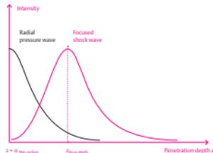
The shock waves have the maximum intensity in the focus (in the depth). The radial pressure waves have the maximum intensity at the point of entry (skin surface).
