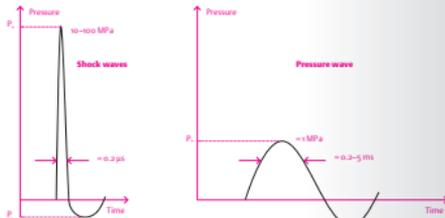
$p_s$  and  $p_p$  are the maximum positive and negative pressure. The amplitude  $p$  of shock and pressure waves differs by a factor of 10-100.
